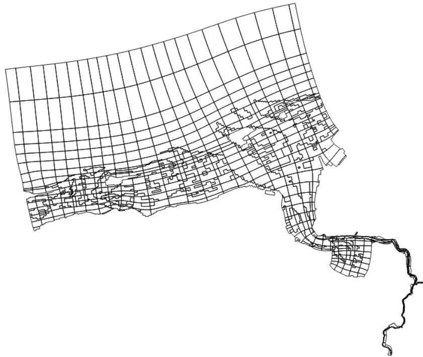
Figure 4.3 Horizontal lay-out of the computational grid for the sediment.
