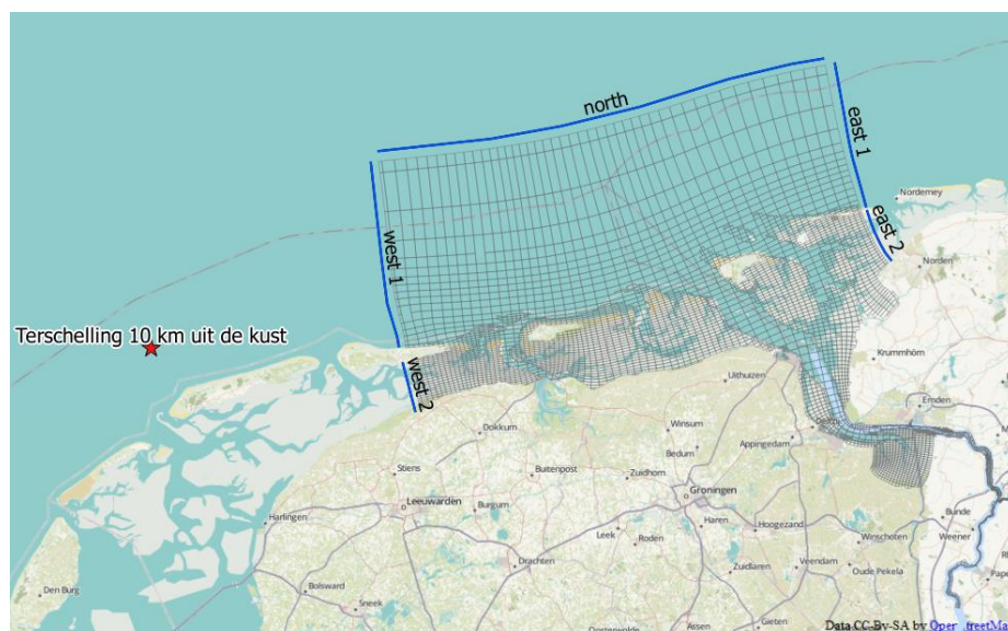
Figure 4.10 Data from the MWTM station "Terschelling 10 km uit de kust" (red star) was used to define boundary conditions.
