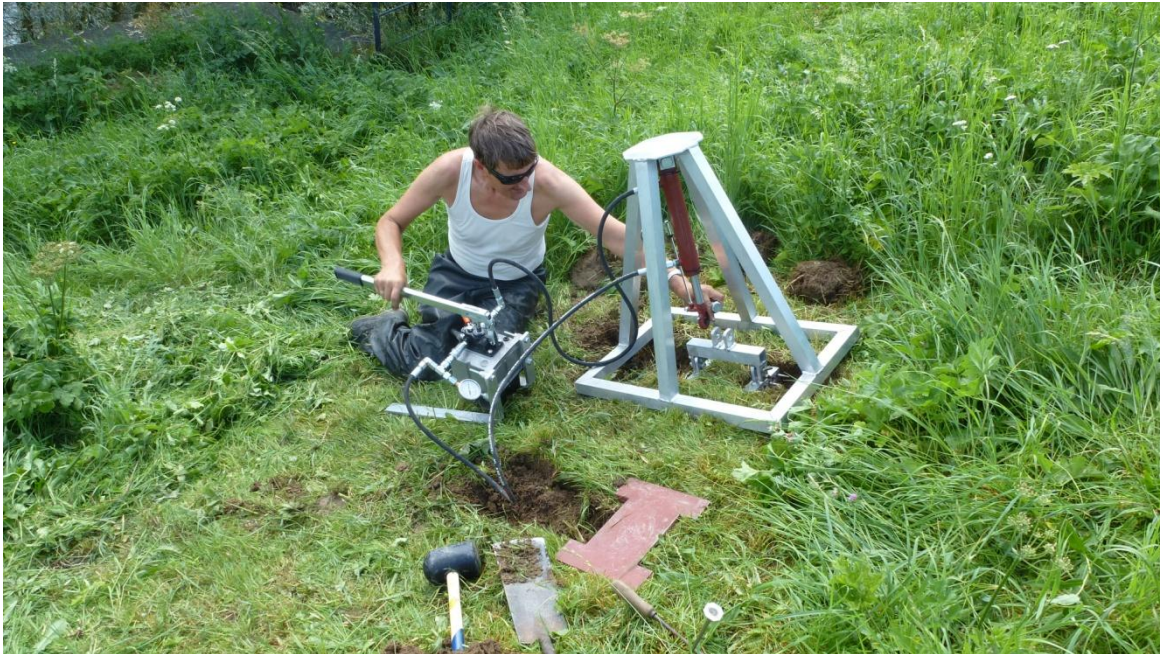
Figure 5.2 Grass sod tensile-stress apparatus
