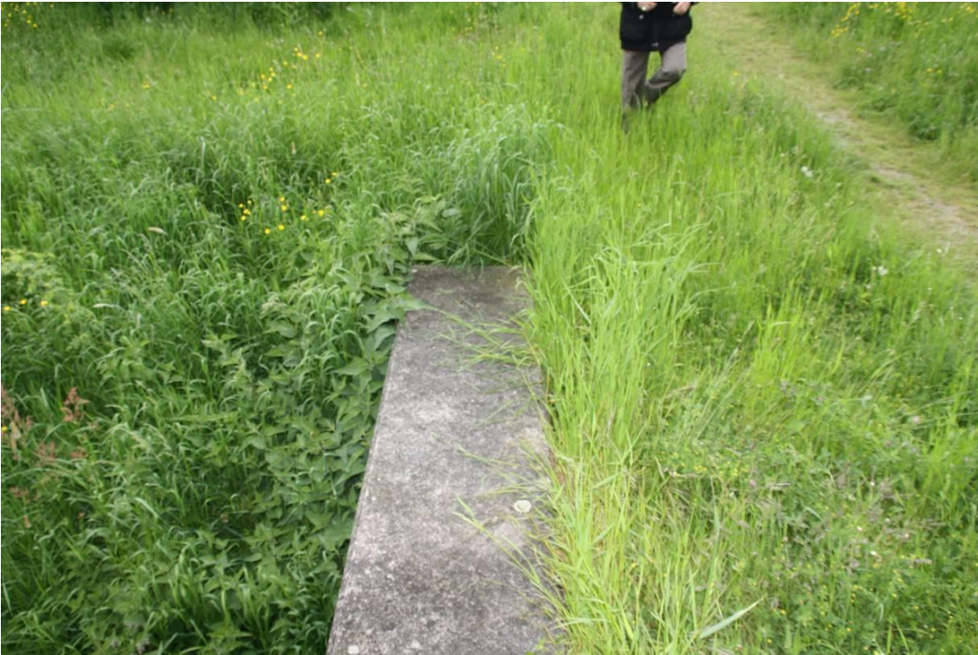
Photo 2.6 Detail of concrete beam. To simulate the erosion of grass near a big obstacle (Location 1) a vertical structure could be positioned (Photo 7)
