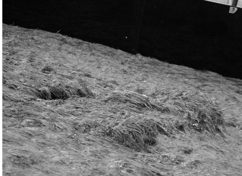
Figure D.2 Instability of grass cover (Bulging-mechanism)
