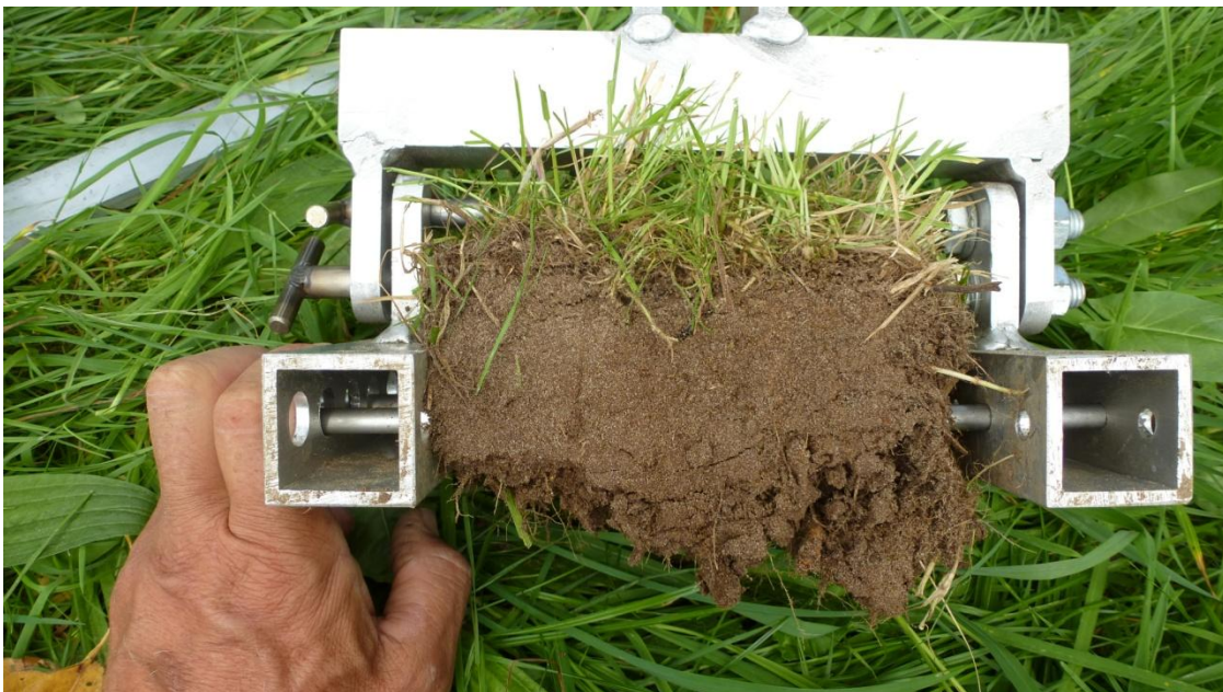
Figure 5.4 Detail of grass sod tensile stress apparatus (thickness of the grass sod is about 5 cm)
