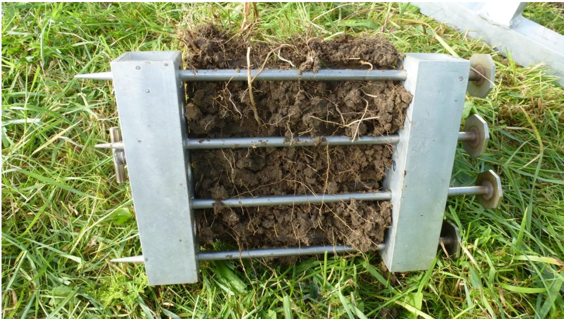
Figure 5.3 Detail of grass sod tensile stress apparatus
