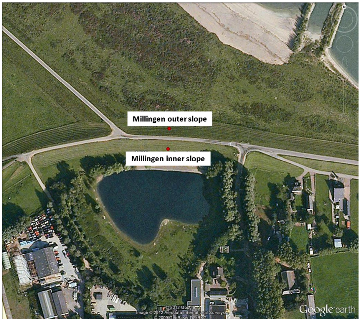
Figure 4.3 Situation of the sampled plots on location 5, west of Millingen aan de Rijn. Each red dot represents a sampling plot that immediately borders the intended wave overtopping test strip and runs parallel to it on the dike slope
