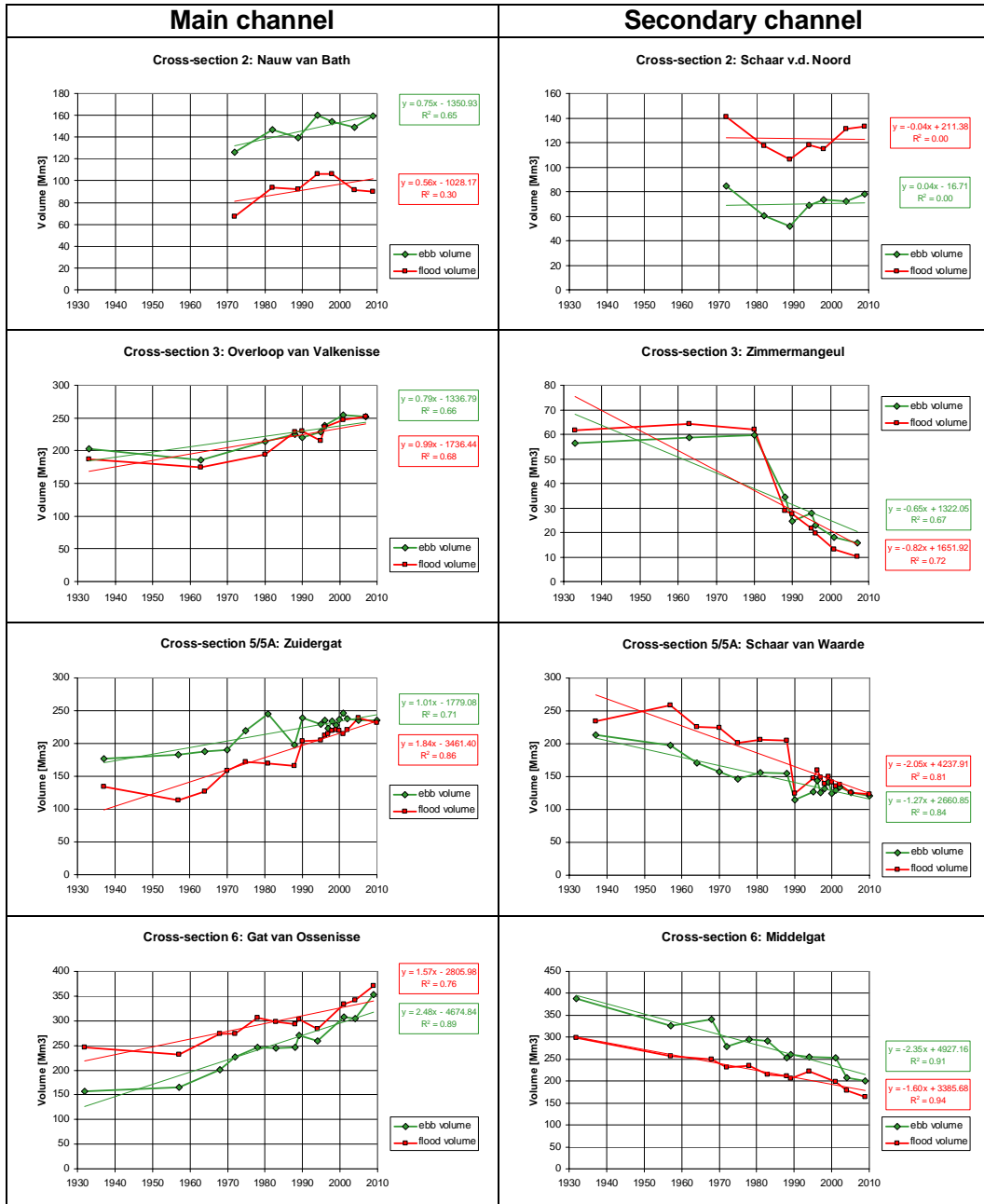
Figure 2.63 shows the ebb and flood volumes for the main channels as well as for the secondary channels.
