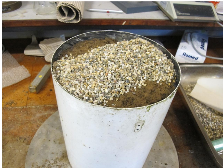
Fig.4 22a Preparing the bottom side by picking off clay parts and application of gravel layer
