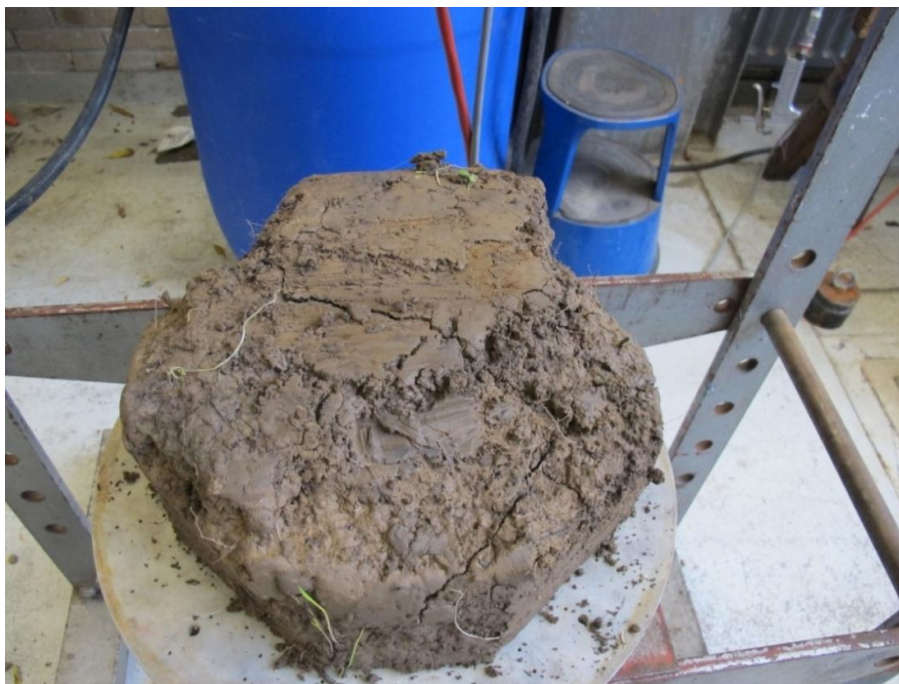
Figure B2 Sod for test 2 with a large fracture on top and the right side
