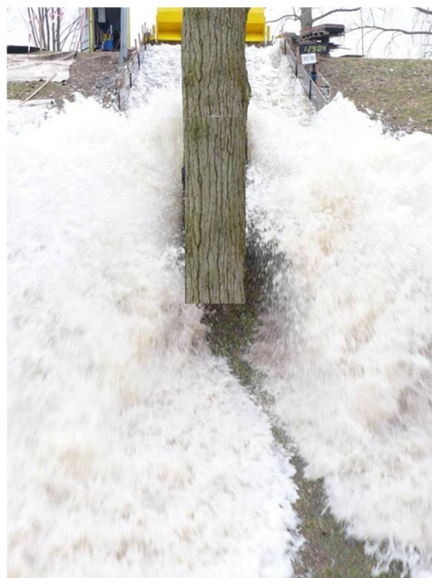
Figure 4.29 Downstream of tree (there is no mixing downstream of the tree) for super critical flow
