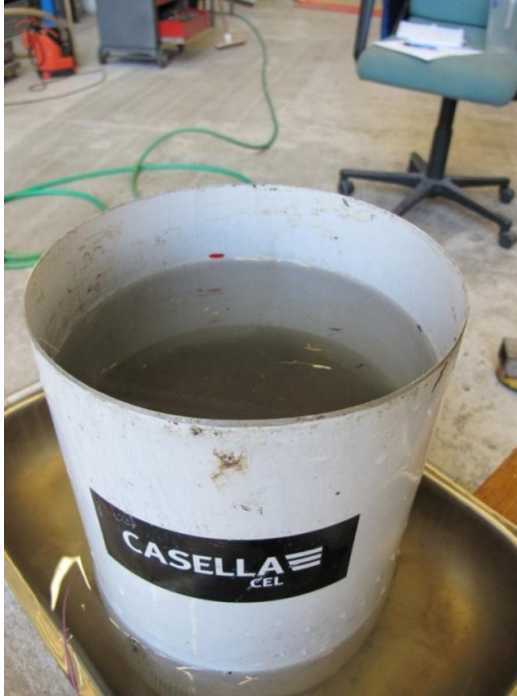
Figure B11 Running falling head test on the first sample
