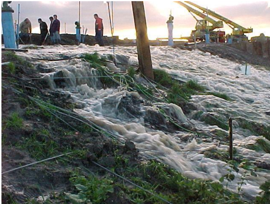
Figure 6.8 Overflow over the landward slope, where no significant erosion (more than 0.2 m deep) occurred during the entire test
