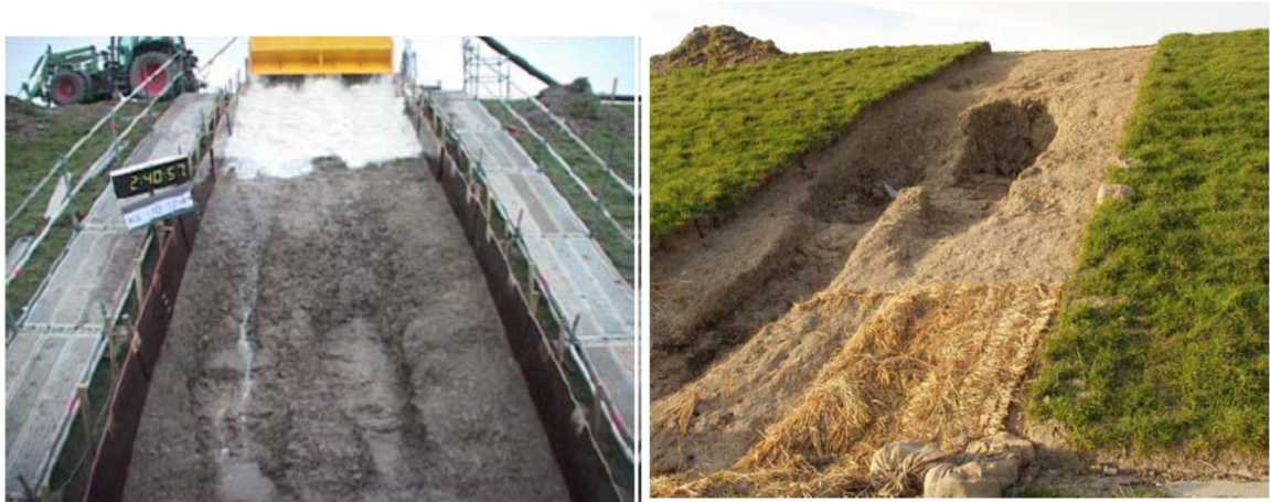
Figure 1.2 Wave overtopping test at Delfzijl where headcut erosion was observed (ComCoast)
