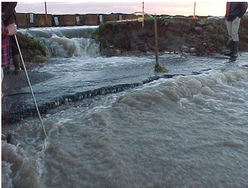
Figure 6.9 The head cut migrates outward, lowering the crest and concentrating the overflow, the scarp deepens into the pavement foundation (sand, caustic lime treated sand, gravel and clay) and undermines the asphalt on the deformed crest
