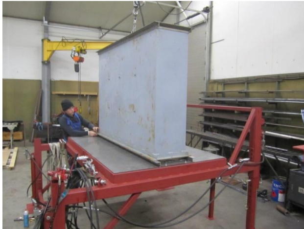
Picture 15. Placing the first module 0.4 m x 2.0 m
