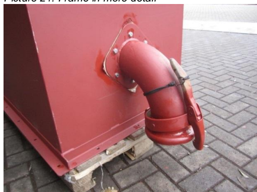
Picture 23. Inlet for pump on upper module
