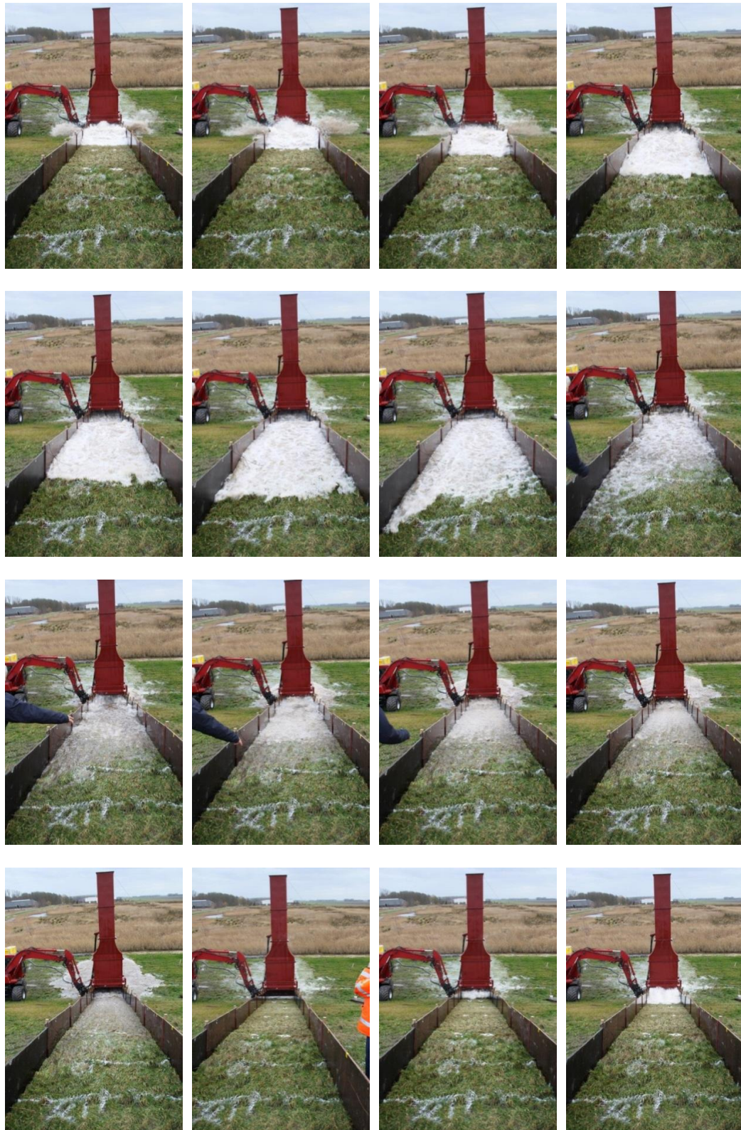
Figure 12. The run-up process for a filling level of 6 m.
