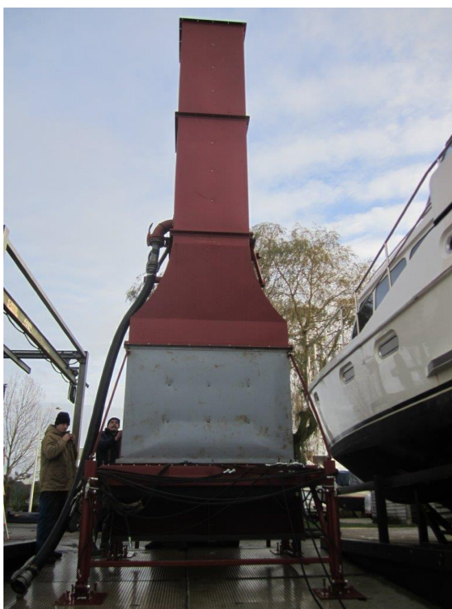
Picture 33. Testing with 7 m water column
