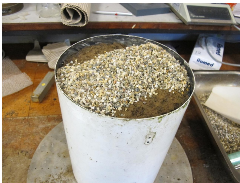
Figure 6.11 Preparing the bottom side by picking off clay parts and application of gravel layer
