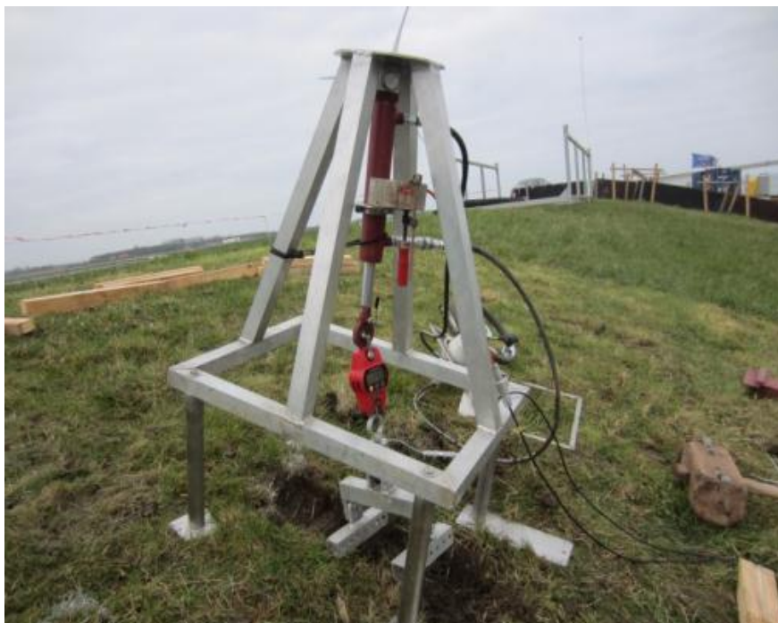
Figure 7.4 Turf-tensile apparatus (pull frame is inside the apparatus)
