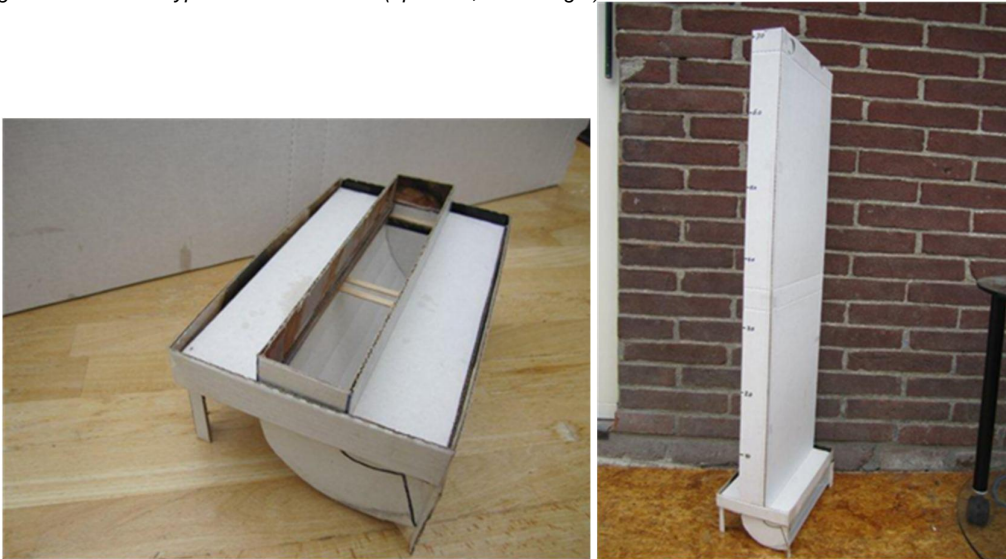
Figure 2.2. The drawer type valve mechanism left with the 110 degree bend. At right the complete machine on a frame with adjustable legs and a height of about 7 m
