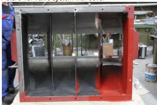
Picture 12. Inner part with guiding plates
