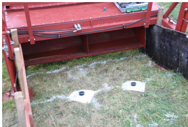
Figure 7. First two paddle wheels 3 cm above soil
