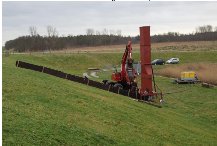
Figure 3. Overall view with measuring cabin, crane, pump, simulator and "flume"
