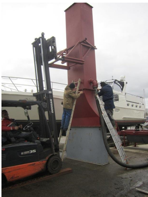
Picture 31. Fixing for 7 m water column testing
