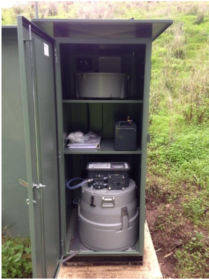
Figure 2.2 Automatic sampler installation (left), and example hydrograph with sample collection times shown (right).
