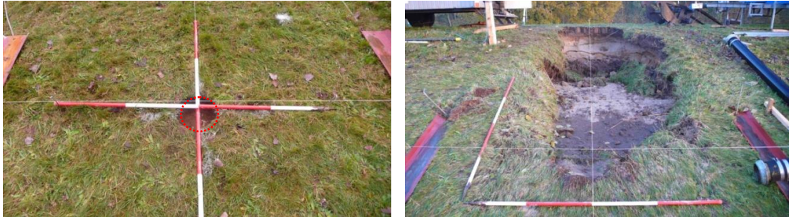
Figure 7. Impression of damage development and initial artificial damage of reference test without transition (Be.1). Artificial initial damage is indicated with a red circle. Left: initial condition, right: after 2234 impacts.
