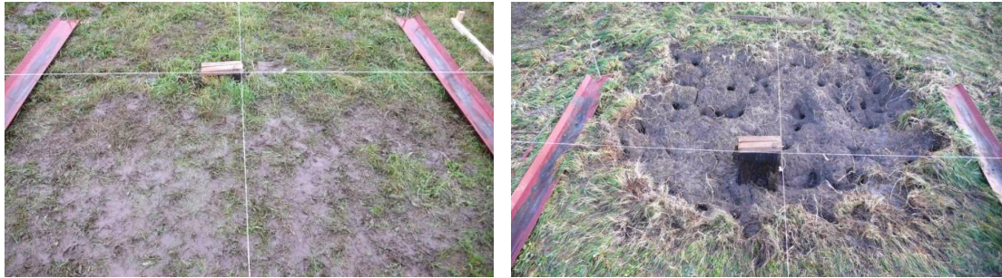
Figure 12. Impression of test with pole (Ha.2). Left: initial condition, right: damage after 2500 impacts.
