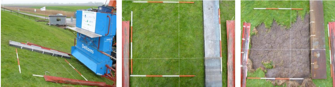
Figure 5. Impression of Test Section Oo.7. Left and middle: initial condition, right: after 5800 impacts of which 1000 impacts were with maximum water level.
