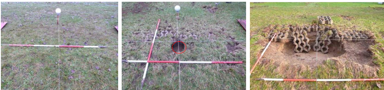
Figure 9. Impression of damage development and artificial damage of Test Section Be.3. Artificial damage is indicated with red circle. Left: initial condition, middle: after 1000 impacts, right: after 4000 impacts.
