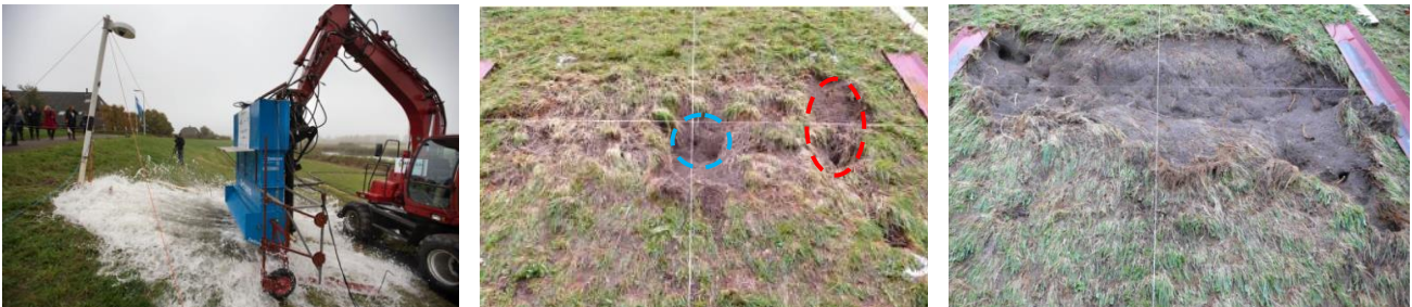
Figure 11. Impression of reference test without transition (Ha.1). Left: during testing, Middle: damage after 2500 impact; the red marker indicates the second erosion hole which is indicated as a separate test section (Ha.4). The blue circle indicates the original location of the artificial initial damage. Right: damage after 6014 impacts.
