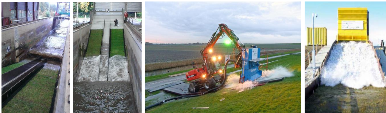
Figure 1. Impression of testing stability of grass slopes with the use of the Deltares Delta Flume (impacts and wave run-up), wave impact generator, and wave overtopping simulator.
