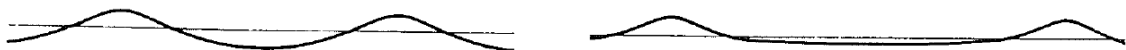
Figure 5.3 Different shape of deep water wave (left) and shallow water wave (right) (Battjes, 1990)
