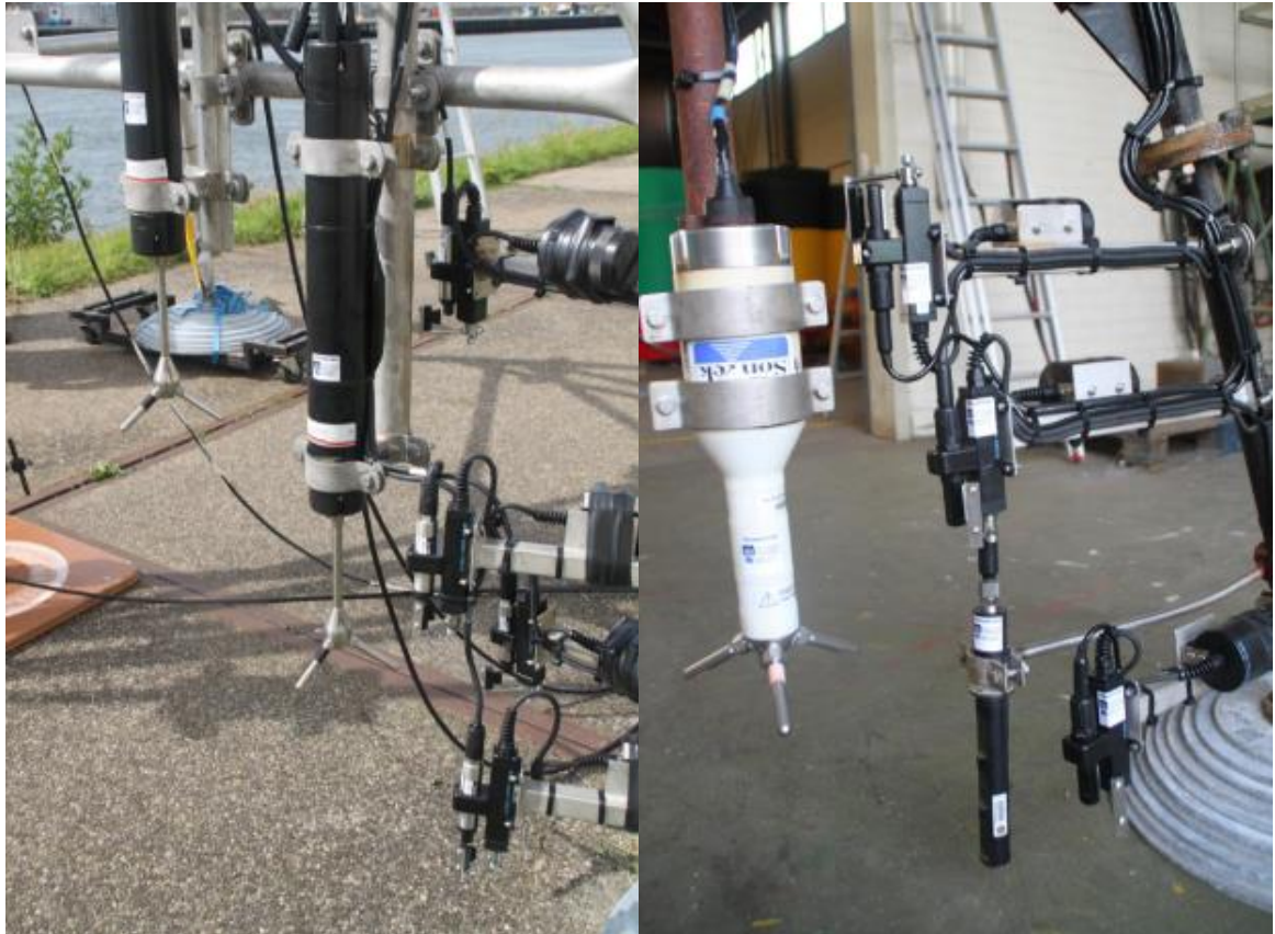
Figure 3.16 Seapoint (left) and Campbell (right) OBSs, installed on frames 5 and 4, respectively.
