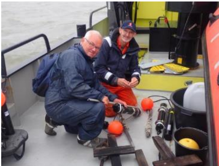
Figure 3.5 ADCPs being prepared for deployment on the watersheds.
