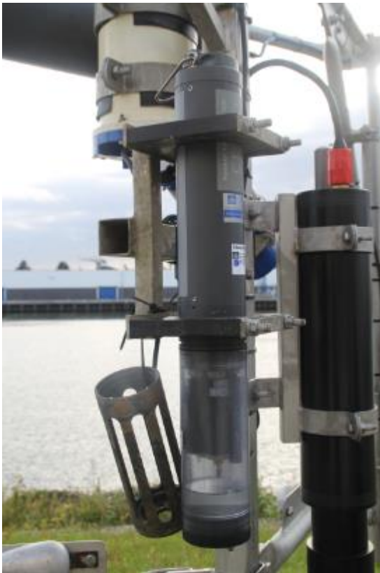
Figure 3.14 YSI 6-Series Multi-parameter Probe (MPP) mounted on Frame 3 (AZG) prior to deployment.
