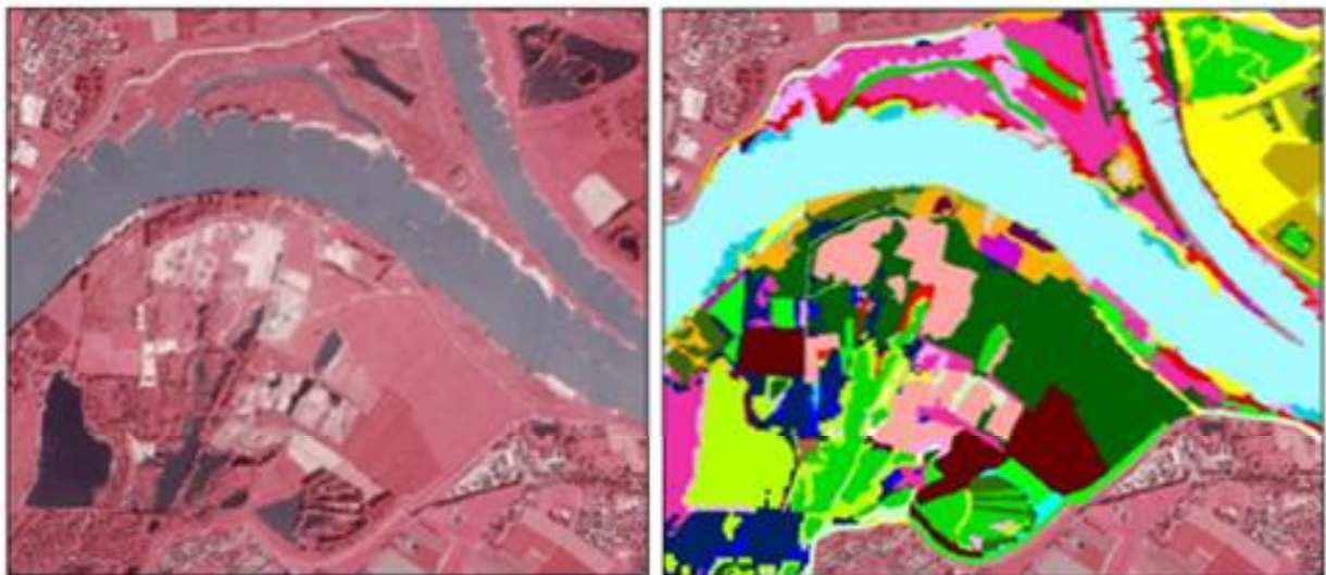
Figure 10 Overlay procedure of the Ecotope map. Five different map inputs are merged into one new map that is classified into ecotopes. (Stehman and Loveland 2005)
