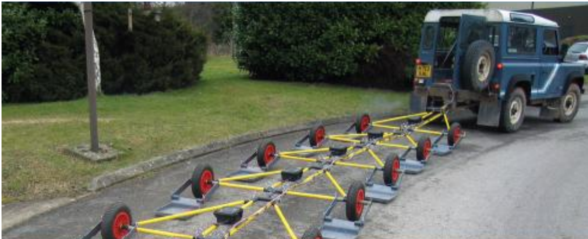
Figure 6 Capacitive sensor towed by a truck. These sensors can be dragged over any surface – due to their capacitive electrical 'connection' with the subsurface they can measure an ERT through surfaces. (Source: British Geological Survey information sheet, see references).
