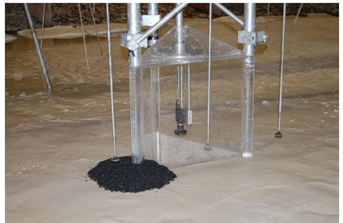
Physical modelling with advanced scour monitoring technique. A video camera is mounted inside the structure and captures images. The scour development can be followed online outside the facility.
