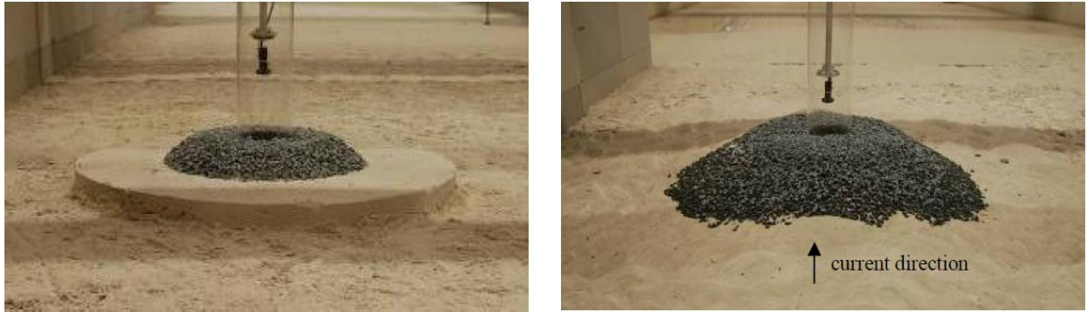
Figure 8.2 Falling apron - illustration of scour protection adaption to seabed lowering. Physical model test from De Sonnevile et al. (2012).
