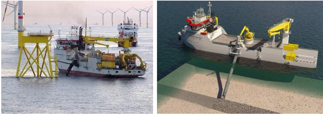
Figure 7.4 Vessel with inclined fallpipe (courtesy of Jan de Nul).
