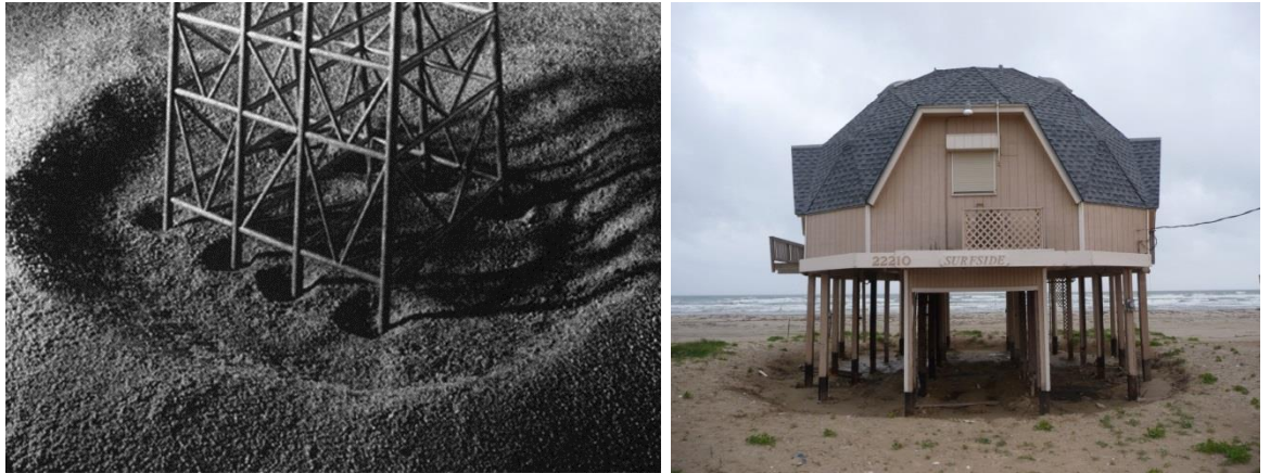
Figure 2.2 (Left) local scour holes around individual jacket legs and global scour pit around entire footprint (Angus & Moore, 1982); (right) local scour holes around foundation piles and global scour hole around beach house after occurrence of Hurricane Ike.
