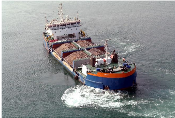
Figure 7.6 Side Stone Installation Vessel (courtesy of Van Oord).
