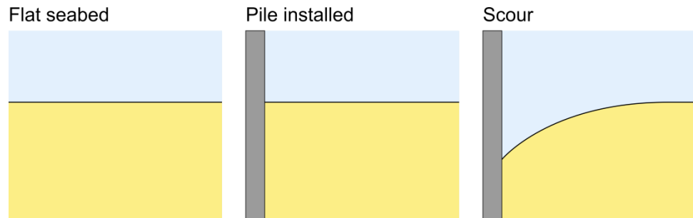
Figure 3.1 Strategy A: No scour protection and allowing free scour development.
