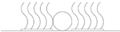
Figure 10.7 Schematic representation of frond mat placement around a cable / pipeline (Source: SSCS).
