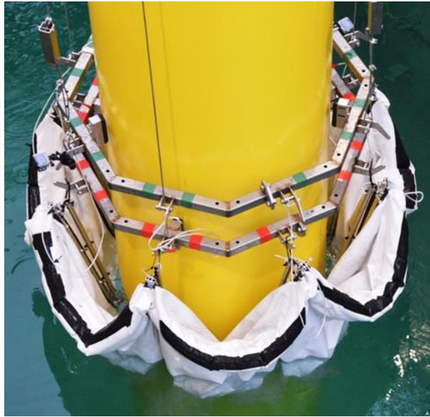
Figure 11.28 Frame with ballast-filled mattresses during model tests.
