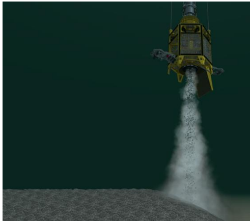
Figure 7.2 Fallpipe ROV (courtesy of Jan De Nul).
