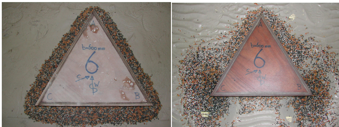
Figure 3: (left) top view of spud can with scour protection before test execution; (right) spud can with redistributed scour protection. The side slopes of the two scour holes at corners B and C are completely covered by protection material.
