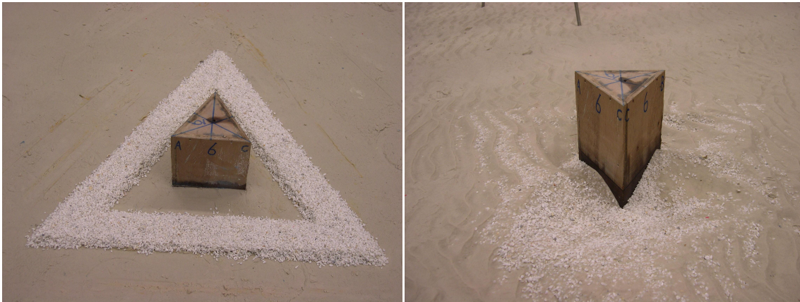
Figure 4: (left) top view of spud can before test execution with scour protection applied at some distance from the spud can; (right) spud can with redistributed scour protection. Due to the redistribution the initial gravel ridges are re-shaped.
