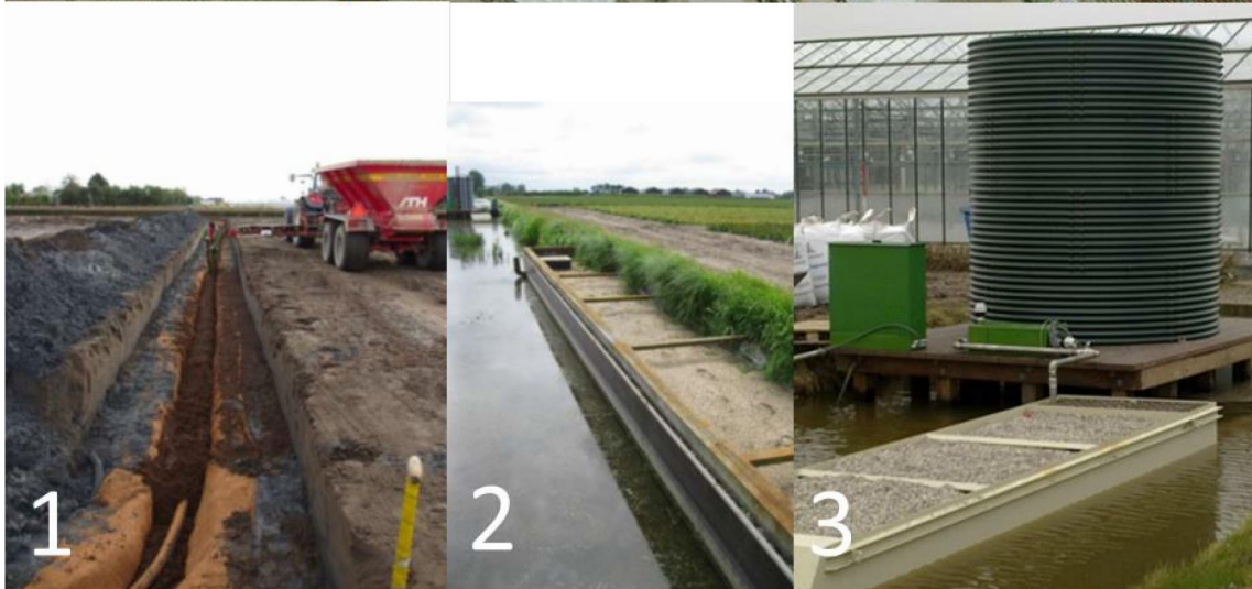
Figure 4. Experimental area. The locations of the field experiments are as follows: (1) Iron-oxide coated sand drains; (2) Canal bank reactor; and (3) Slow sand filter at the end of the drainage canal.
