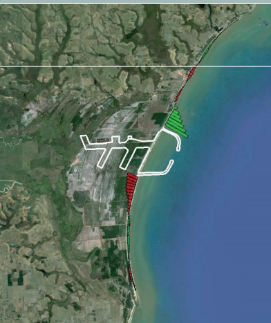
Model output showing erosion (red) and accretion (green). The bars are exaggerated to make the patterns clearer.
