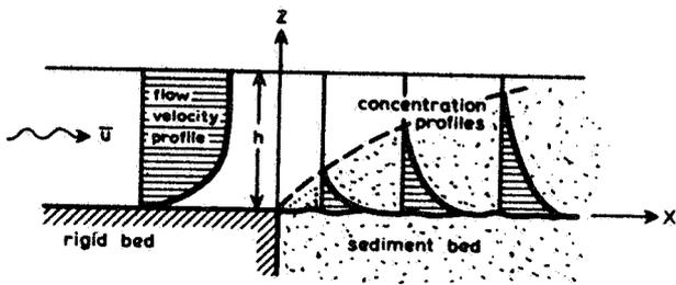
FIG.1 FLOW, INITIALLY FREE OF SEDIMENT, OVER A SEDIMENT BED
