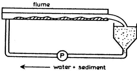
FIG. 1 SAND-RECIRCULATION SYSTEM
