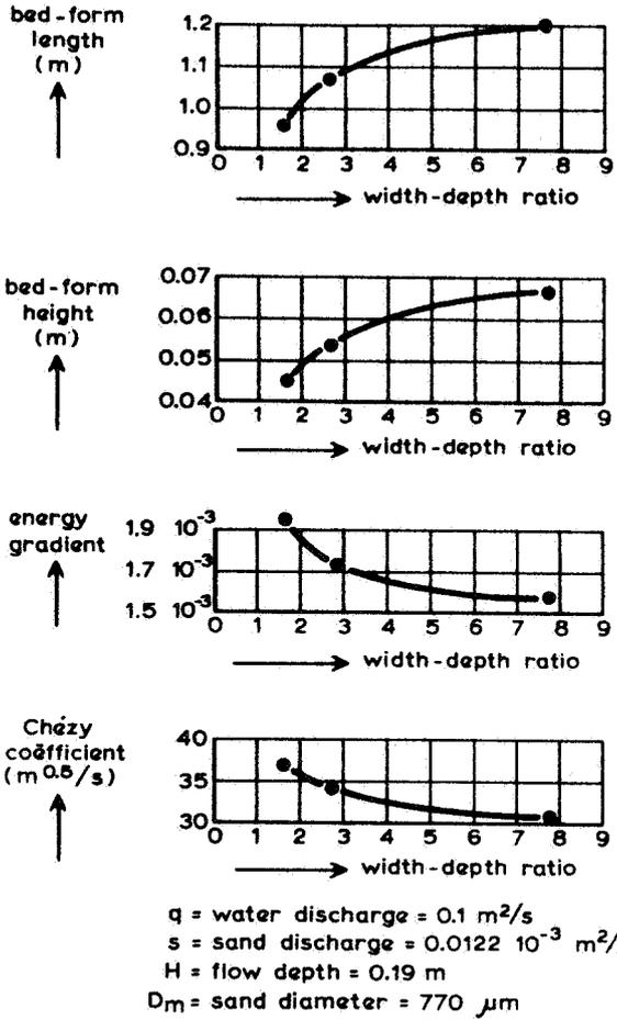
FIG. 6 BED-FORM DIMENSIONS IN MIDDLE PROFILE, ENERGY GRADIENT AND CHÉZY-COEFFICIENT AS A FUNCTION OF FLUME WIDTH
