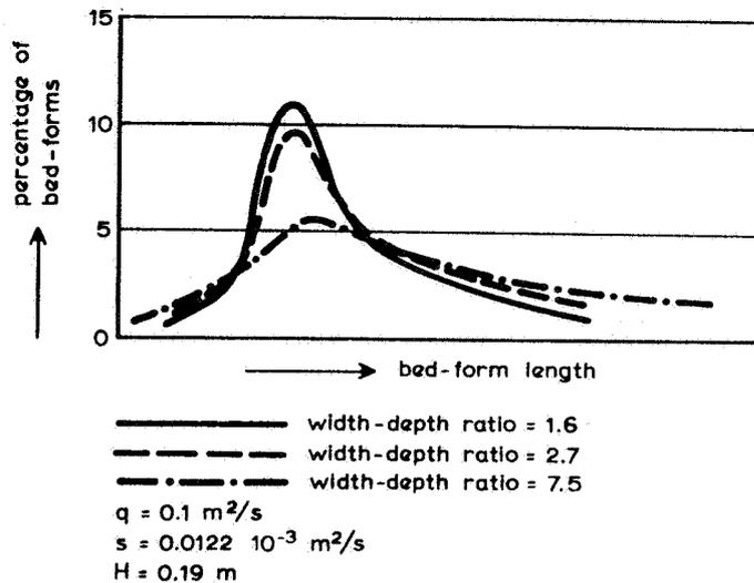
FIG. 7 PROBABILITY DENSITY FUNCTION OF THE BED-FORM LENGTH IN MIDDLE PROFILE
