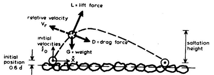
FIG.2 TRAJECTORY OF A SALTATING PARTICLE
