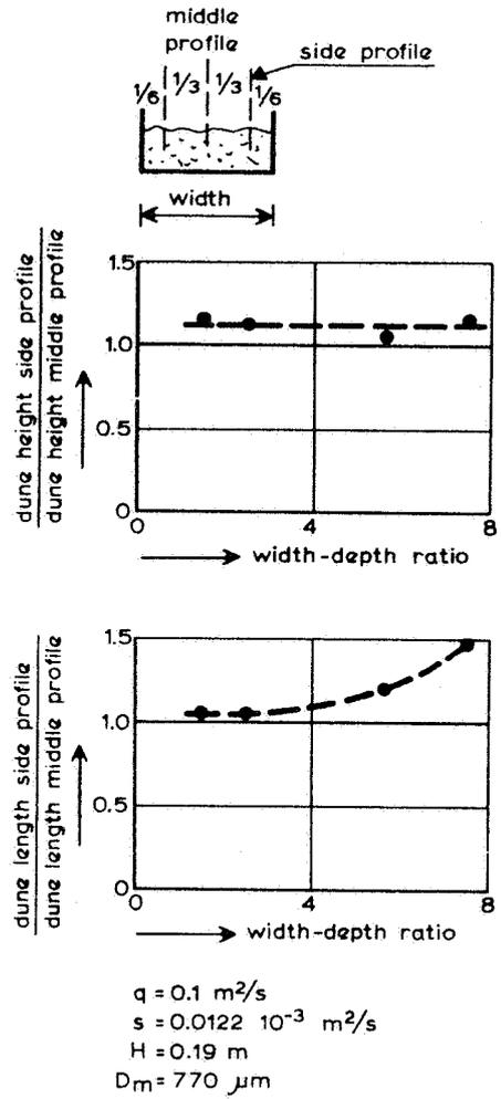
FIG. 8 RATIOS OF BED FORM LENGTH AND HEIGHT IN MIDDLE AND SIDE PROFILES AS A FUNCTION OF FLUME WIDTH
