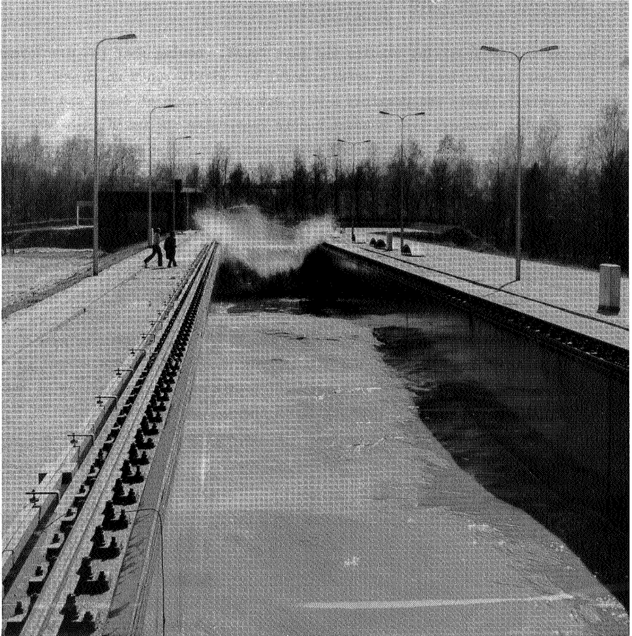
Fig. 7 Delta Flume breaking wave, test 5 (photograph)
