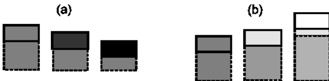
Figure 2.8. Transport layer concept in Delft 3D. (a) Erosion of a cell (b) Sedimentation in a cell. The solid lines represent the active layer and dotted lines the sediment layer. Darker colours are coarser sediments (Dastgheib, 2012).
