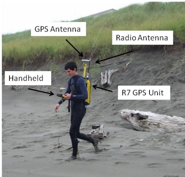
Figure 4. Topographic surveys use a handheld data logger to navigate while the GPS acquires position information. The radio antenna enables GPS communication with the base station. A measurement of the height of the GPS antenna for each operator is required to correctly record the elevation of the beach surface.
