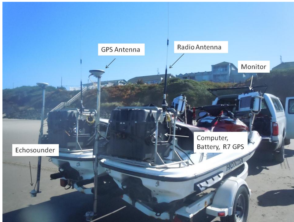
Figure 2. The CPS equipment set up for data collection includes a watertight case, monitor, echosounder, GPS and radio antennas. The case holds a small computer, the echosounder electronics, a Trimble R7 GPS unit, and a battery. Waterproof cables connect the equipment inside the case to the equipment mounted on the outside of the boat. The echosounder transducer and GPS antenna are rotated to a horizontal position during travel in shallow water to prevent the transducer from being damaged. The radio antenna allows the R7 rover unit to communicate with the base station. The monitor displays the transect, position and speed of the boat, and GPS status, enabling the CPS operator to maintain an ‘on line’ position as well as verify GPS and echosounder status during the survey.
