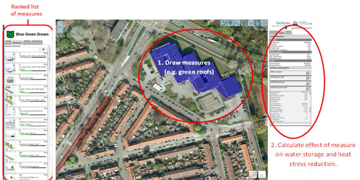
Figure 5.2 AST calculates the effectiveness of the measure for water quantity regulation (reduction of runoff) and reduction of heat stress ( http://bgd.org.uk/tools-models/ ).
