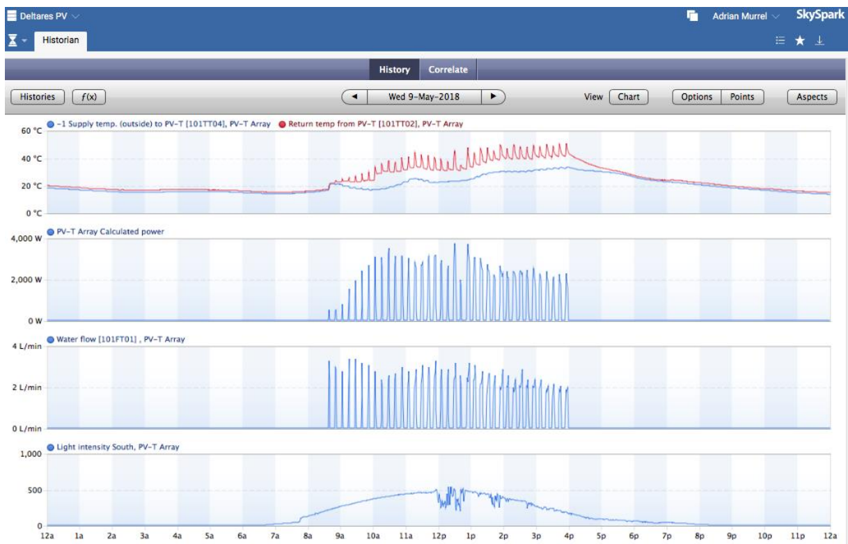
Figure 10. Thermal output data from the phase 1 (10 collector) Virtu solar array: 9-May-18.
