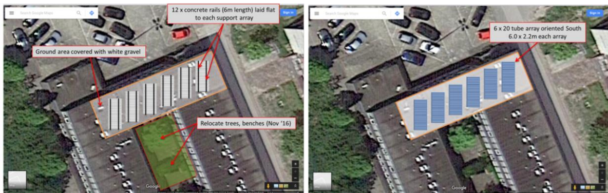
Figure 5. Placement details of Virtu panels
