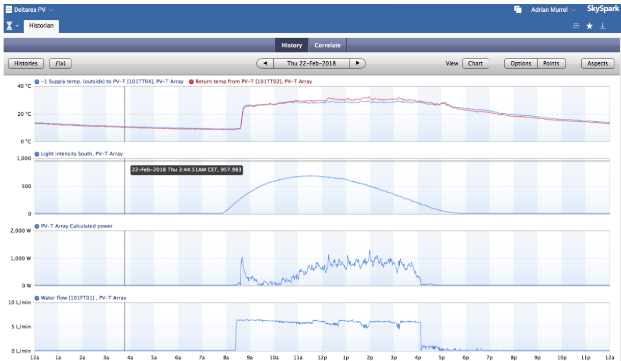
Figure 9. Thermal output data from the phase 1 (10 collector) Virtu solar array – 22-Feb-18
