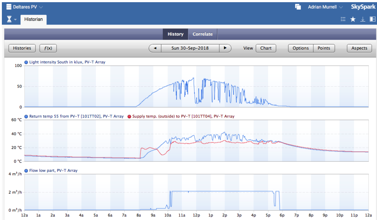
Figure 13. Performance data from the Virtu solar array on a partially cloudy day
