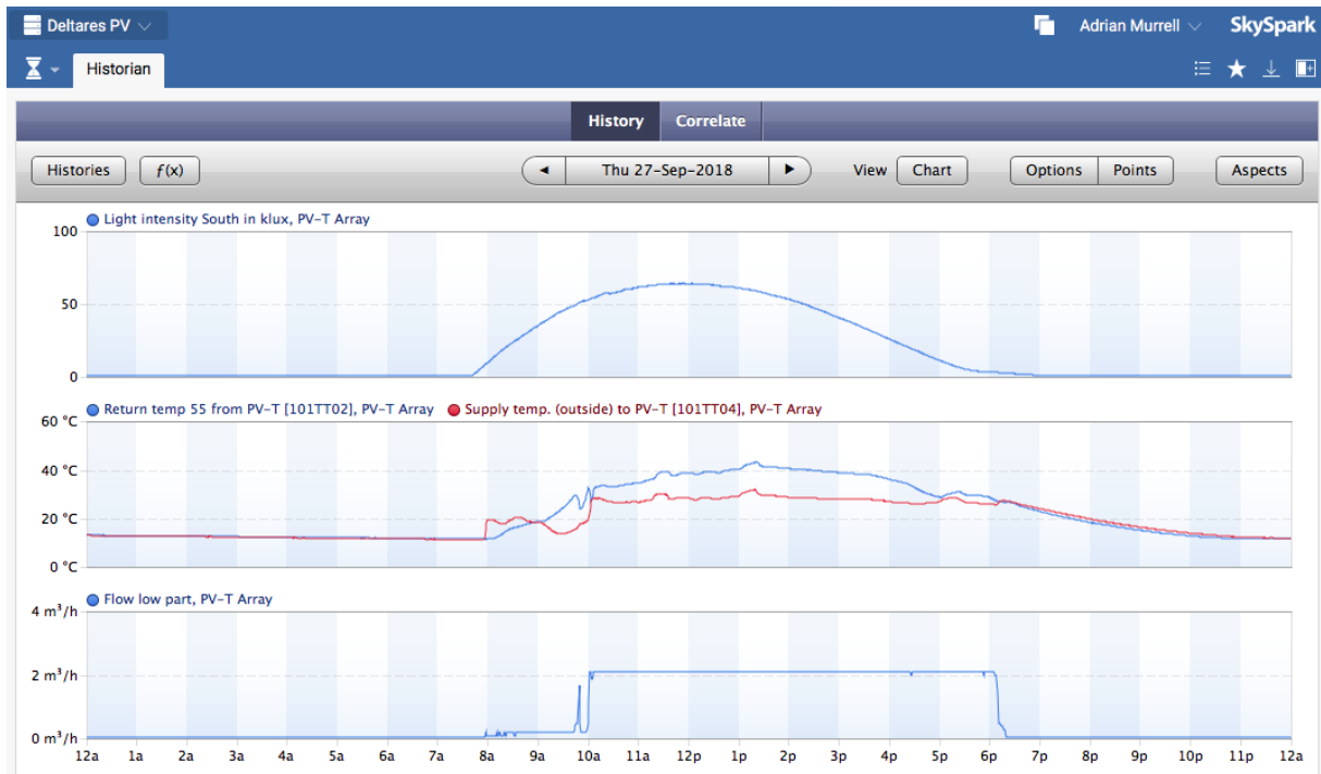
Figure 12. Performance data from the Virtu solar array on a clear sunny day
