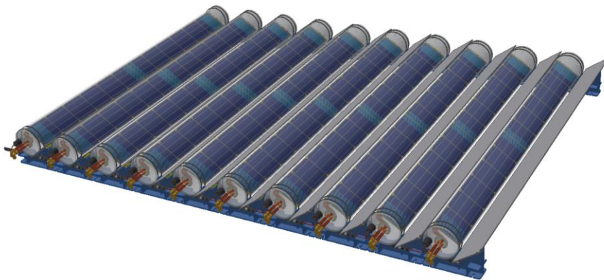
Figure 1. Schematic representation of Virtu PVT panel
