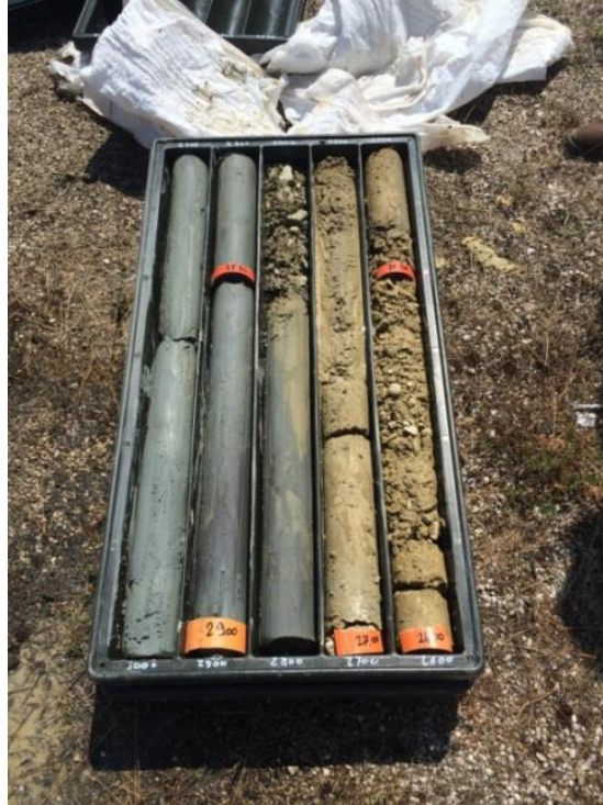
Figure 12. Picture of samples taken from 26 meters' depth up to 30 meters' depth in the first borehole.
