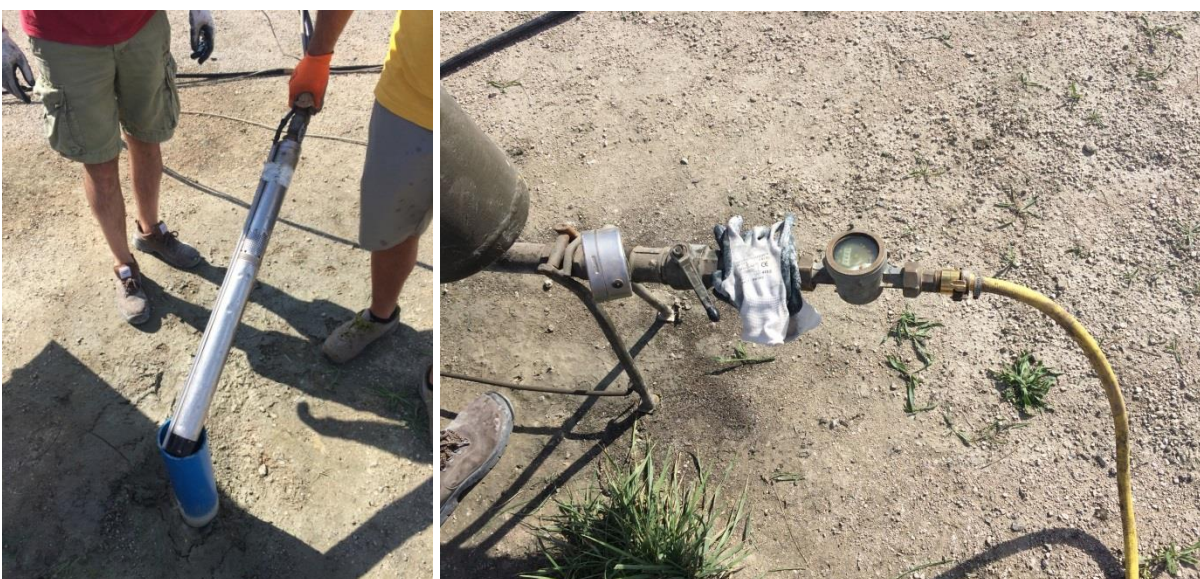
Figure 18. Picture i) of the water pump and ii) of the water volumetric flowrate meter.
