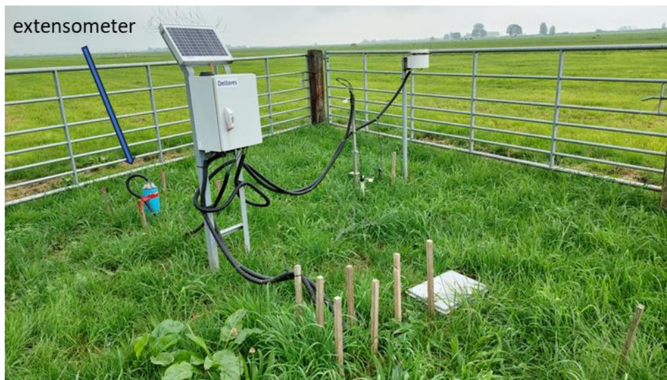
Figure 1: Field plot with extensometer at land subsidence monitoring site Berkenwoude.
