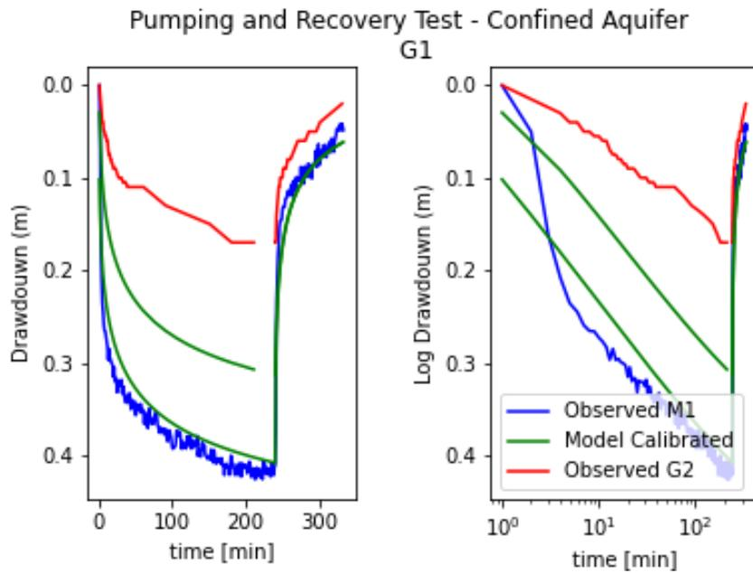
Figure D Measured drawdown and recovery and model fit for M1 and G2. The blue line shows the measured data by a sensor in the monitoring well M1. The red line shows the manual measurements conducted in the well G2, and the green lines show the results of the model when calibrating it for M1 and G2 combined.
