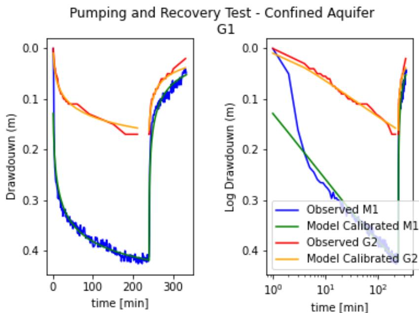
Figure C Measured drawdown and recovery and model fit for M1 and G2. The blue line shows the measured data by a sensor in the monitoring well M1. The red line shows the manual measurements conducted in the well G2, and the green and orange lines show the results of the model when calibrating it separately for M1 and G2.
