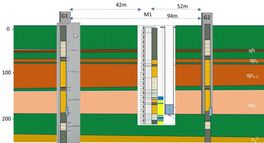
Figure B Cross-section showing the location, lithology and design of G1, G2 and M1 in the Nga Bay site. The layers in the cross-section representing the aquifers and aquitards are the result of the interpolation of available wells in the region.
