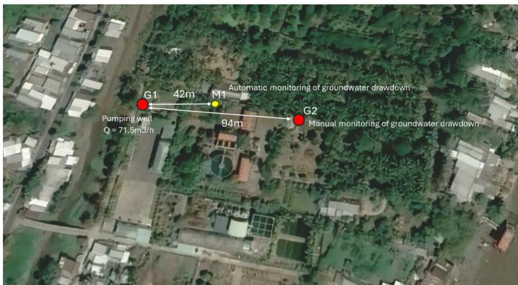
Figure A Map with the wells used for the pumping test
