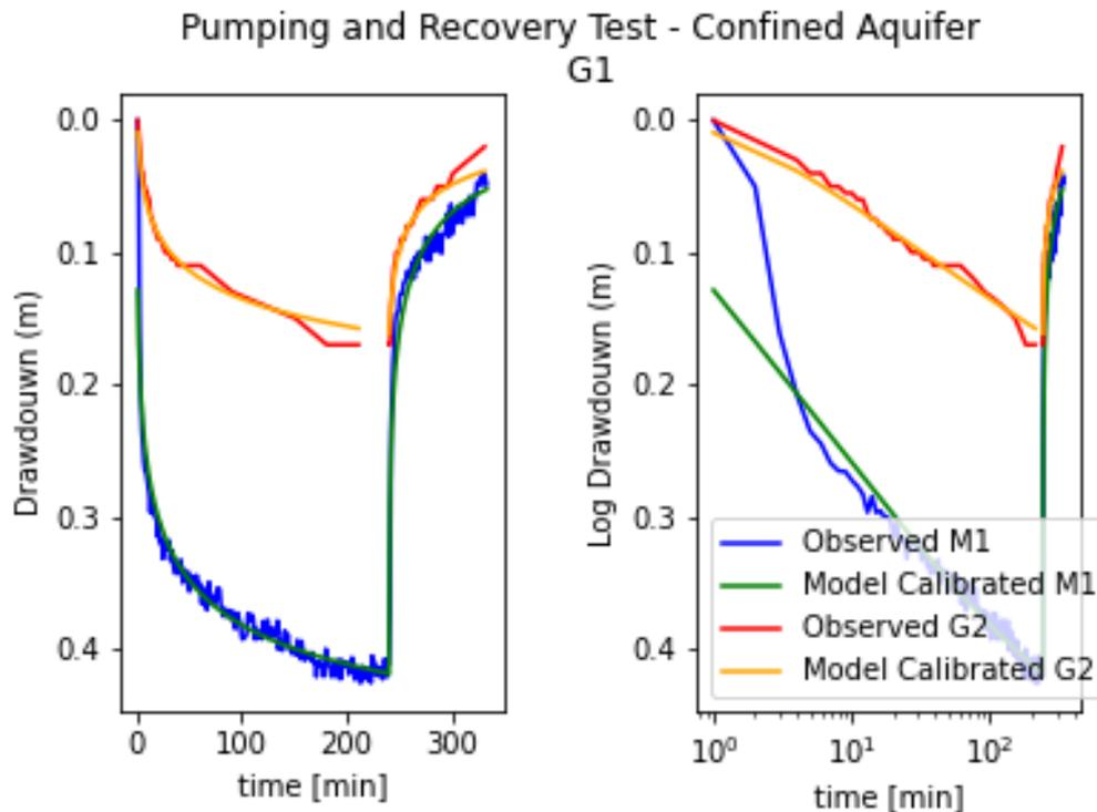
Figure 3: Measured drawdown and recovery and model fit for M1 and G2. The blue line shows the measured data by a sensor in the monitoring well M1. The red line shows the manual measurements conducted in the well G2, and the green and orange lines show the results of the model when calibrating it separately for M1 and G2.
