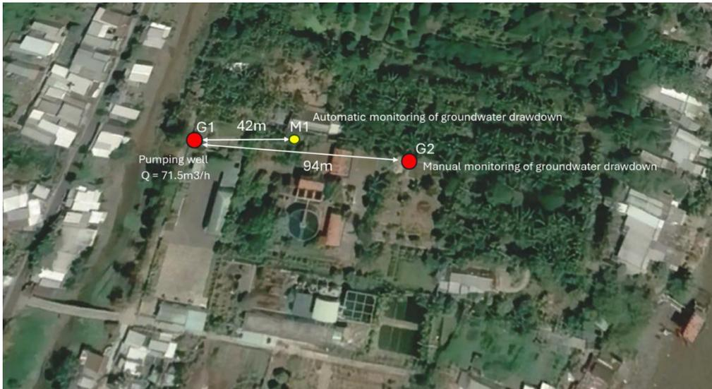
Figure 2 Map with the wells used for the pumping test
