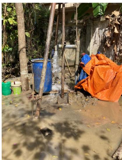
Figure 1: Capacity measurement with barrel
