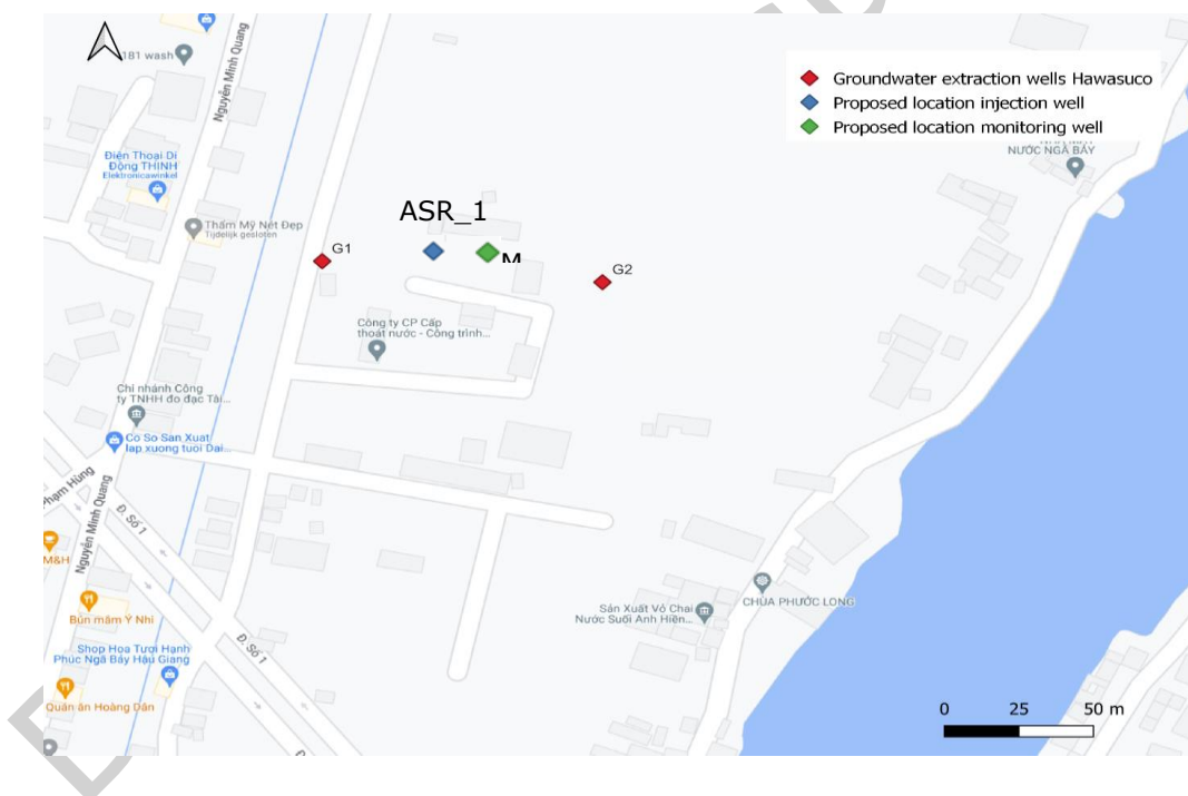
Figure 10: Location for the ASR well between the existing extraction well G1 and the new monitoring well M_1
